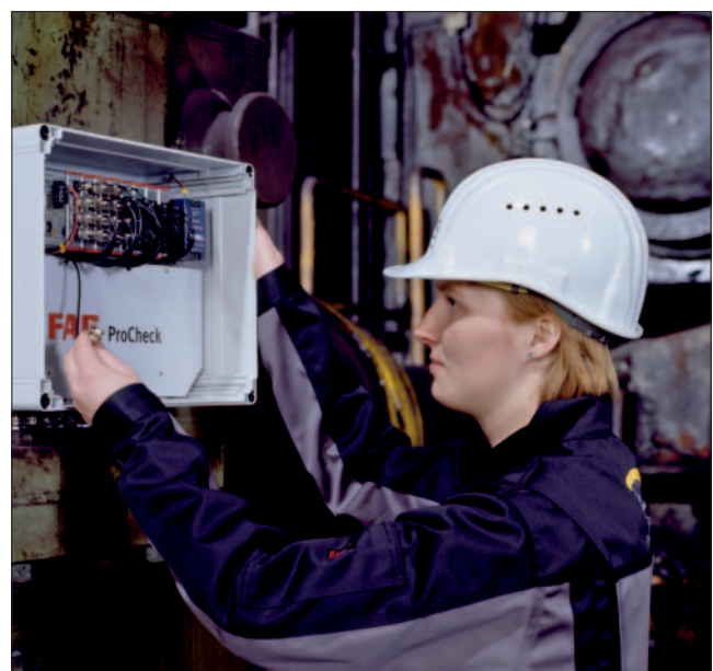
Gearbox monitoring on a hot rolling line
